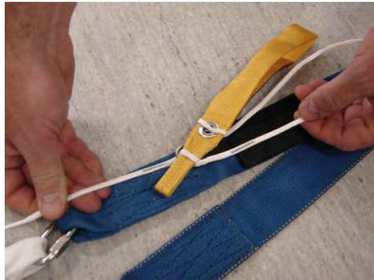
4. S fold the excess control line. Secure the toggle and excess control line according to the instructions of the harness manufacturer.
