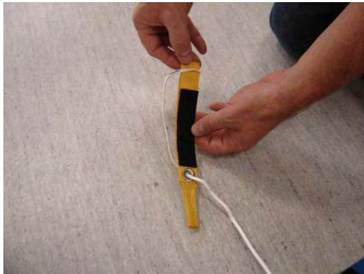
6. Pull all excess line through the toggle until the loop is taut.
